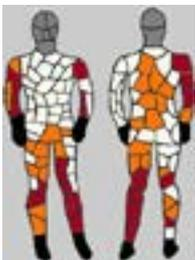
This test produces a body map showing predicted 2nd and 3rd degree burns and so indicates how effectively a garment protects the wearer.
